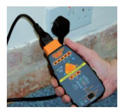
Your tester is equipped with 2 methods of connecting to a socket or a spur. This test lead is used for sockets.
