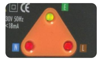
This is an example of 'Fault Locate' showing Live (Phase), neutral reverse.
